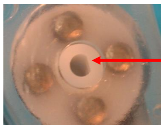
Verdrehschutz / Anti-twist guard
